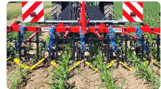
8-row hoeing system for maize, with side shifting frame and fingerweeder 37 cm, yellow
