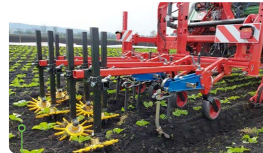
4-row parallel sliding system with yellow fingerweeder 31 cm, yellow in Chinese cabbage
