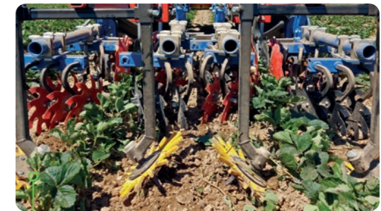
2-row strawberry hoe, combination of star cultivator and fingerweeder 37 cm, yellow
