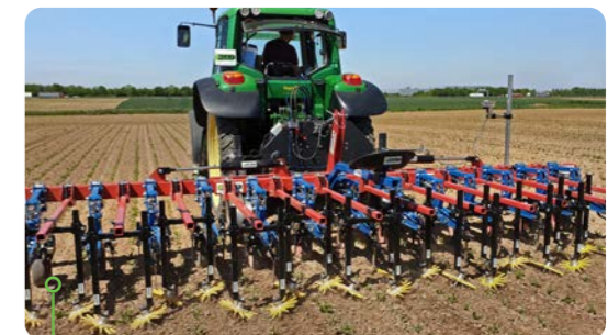
12-row hoeing system for corn, with side shifting frame and fingerweeder 37 cm, yellow
