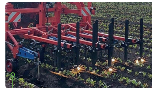
4-row parallel sliding system with yellow fingerweeder 31 cm in beet
