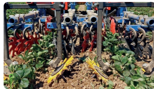
2-row strawberry hoe, combination of star cultivator and fingerweeder 37 cm, yellow
