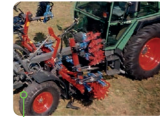
Star-Cultivator, 4-rows in the Fendt GT 275 for strawberry cultivation Spring-loaded tool support with tendrillar cutting discs, 10 stars per row.
