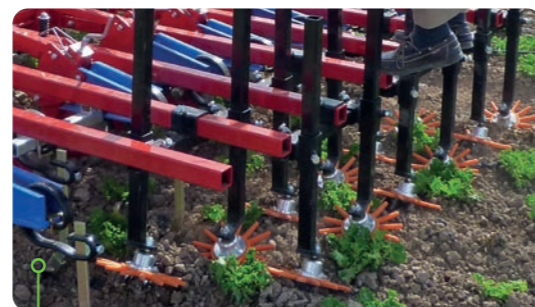
8-row chopping system for lettuce with manual control and fingerweeder 31 cm, orange
