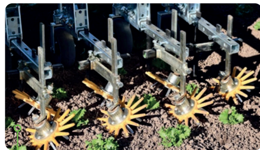
The small yellow fingerweeder with 24 cm diameter, used in the Naio robot for cultivating lettuce
