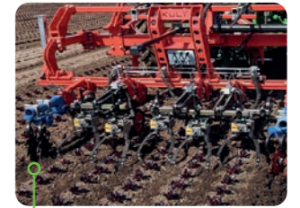
Star-Cultivator as lane-loosener Parallelogram-guided tools with pre-loosener, 2 stars at each side.
