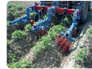
Star-Cultivator, rear mounted, 2 rows for potatoe cultivation Parallelogram-guided tools with pre-loosener, ridge-tine-harrow, mechanical self-guidance 4 stars per row.
